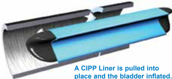
After curing the bladder is removed leaving behind a "pipe within a pipe".
