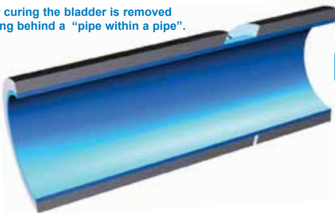
A CIPP Liner is pulled into place and the bladder inflated.
